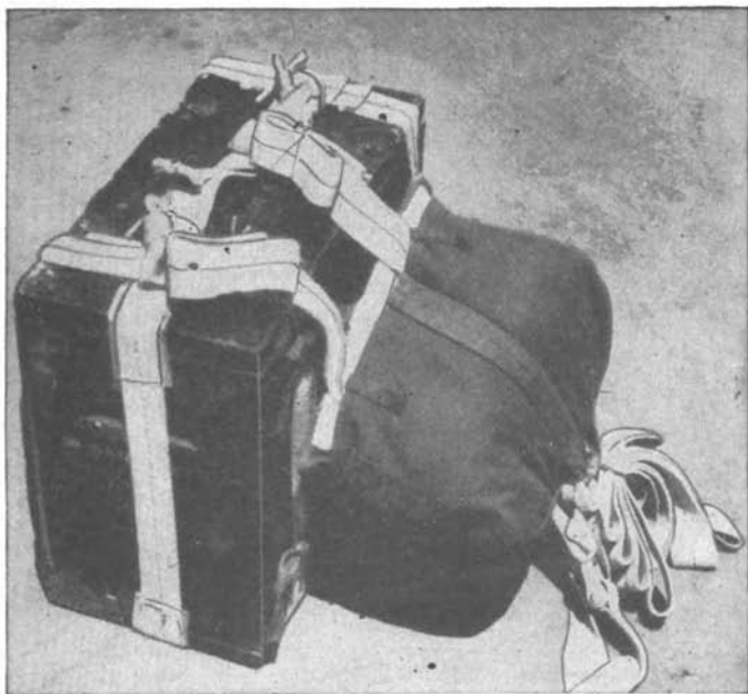
FIGURE 8.—Type A-7 ammunition delivery unit with canopy in pack preparatory to dropping.
