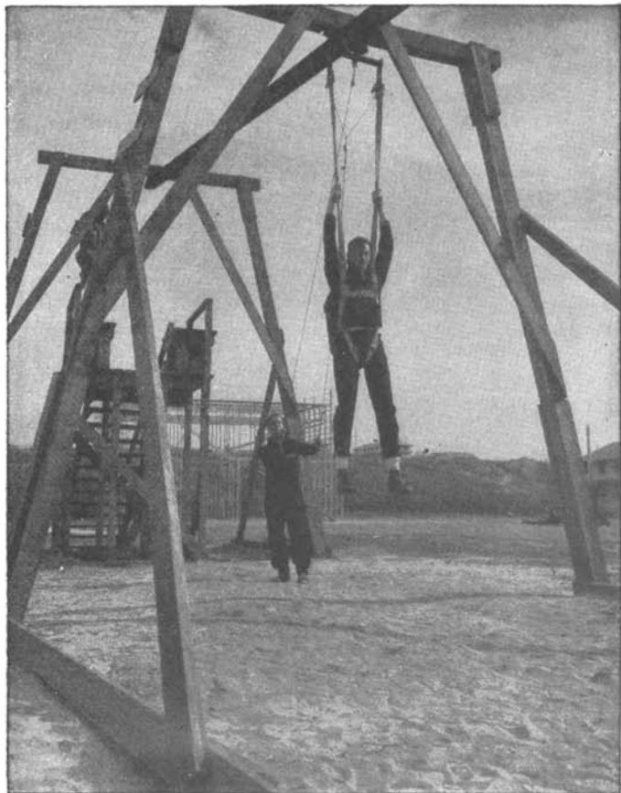
FIGURE 26.—Parachutist sliding down inclined beam of landing trainer. Instructor holds ropes tied to release mechanism.
